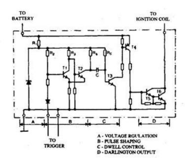
Magnetic coil driver circuit
